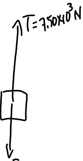
$$F_g = (7.00 \times 10^2 \text{ kg})(9.81 \text{ m/s}^2)$$
